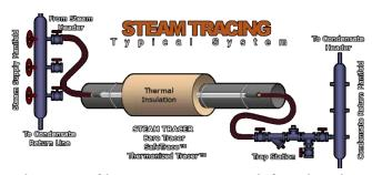
The practice of heating a pipe as materials flows through it to keep the materials at a constant temperature and compensate for heat loss is known as heat tracing.
